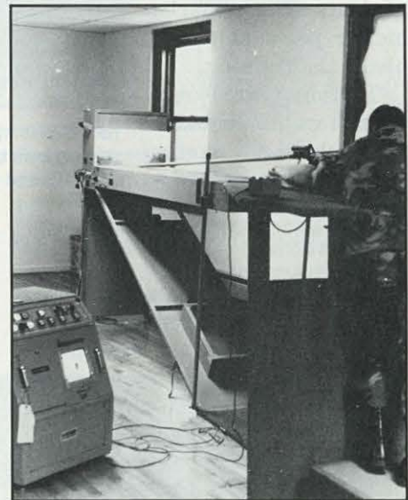
Above: A video screen on the weaponeer's control panel shows where the bullet hits the target and where the aiming point was. Top: Spec. Kim Howard sights down the barrel of a M16 attached to the Weaponeer.
