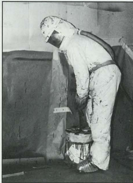
ABOVE: Sgt. Howard Behlmer (left) and Pfc. Michael Vantilburg prepare a 6.2 liter engine for a dynamometer test. RIGHT: Spec. George Oliver mixes a new batch of CARC radar resistant paint.
