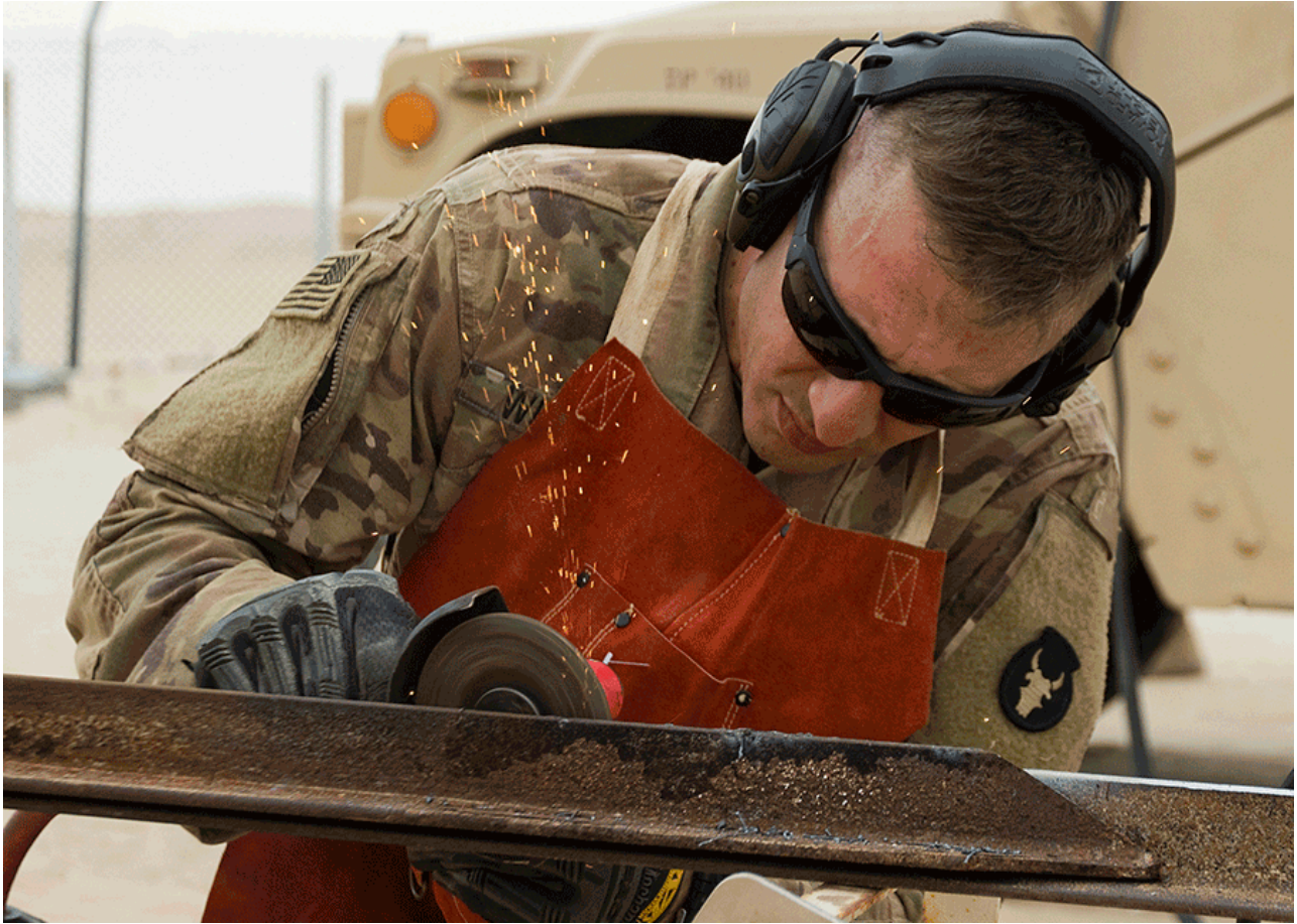
2019 ~ Sgt. 1st Class Justin Whale, maintenance platoon sergeant with Company H, 134th Support Battalion, Task Force Spartan, grinds a fresh weld on a pullup bar during joint exercise Iron Union Dec. 7, 2019, near Abu Dhabi, United Arab Emirates. Iron union is a recurring, bilateral exercise between TF Spartan and the United Arab Emirates Land Forces.
